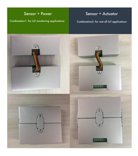
[Note: Use 6 pins female-2-female connector to connect your nodes guided by male headers on both side of individual units]
